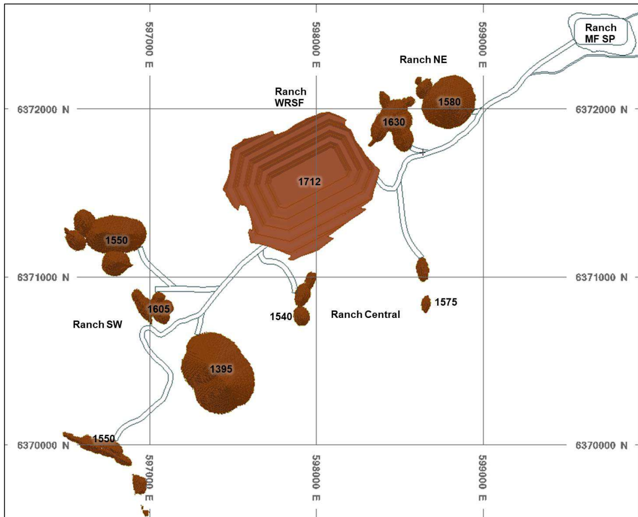
Figure 16-27: Ranch Area Pits and WRSF Status at End of Year 14 (LOM)
